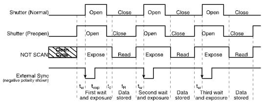
Figure 18. Timing Diagram for External Sync Mode (- edge trigger)
